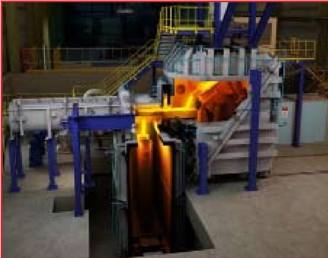
Consarc designs all VIM furnaces such that the pouring is accomplished by inserting a tundish in line with the direction of pour, not perpendicular to the direction of pour, and without the use of a launder, as is required in tilting chamber type systems (VIDP). This significant design criteria means that Consarc VIM furnaces have the following advantages:
