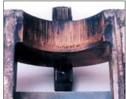
Fig. 6 — The horseshoe-shaped portion of this single-shot (channel) coil has numerous scratches resulting from improper locating of a splined shaft in the heating position. As a result, coil life was dramatically reduced.
