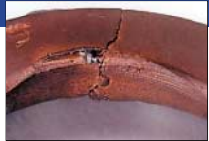
Fig. 5 — Severe damage to this coil's inside diameter resulted in abnormal current flow, a decrease in mechanical strength at the damaged area, and eventual fracture.
