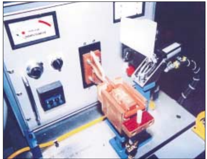
Fig. 3 — An Inductoheat system for adhesive bonding a rubber gasket to a metal brake pedal support. The operation takes just 4 seconds, using a 2 kW, 30 kHz inverter.
