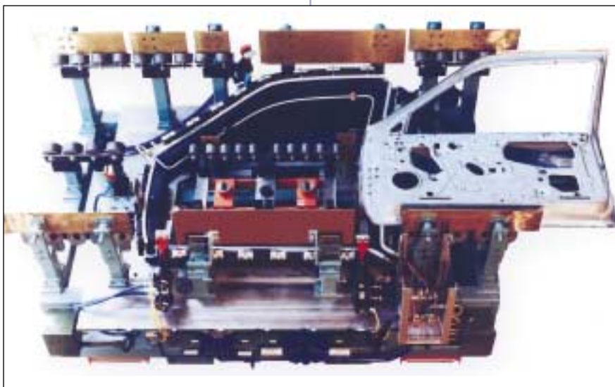
Fig. 4 — Fixture for full- or partial-periphery cure of adhesive hem bonds in automobile door panels. Note panel lifting mechanism. Photo courtesy Inductoheat.
