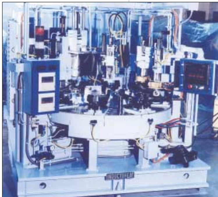
Fig. 1 — Eight-station shrink fitting machine is used to assemble truck steering knuckles. The Inductoheat system produces 30 knuckles per hour.
