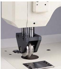
Alleman says, “The SeamMaster™ has a higher clearance between the wheel and the horn than do traditional sewing machines. As a result, it is ideal for hand-guided applications with tight tolerances, as well as for working around curves.
