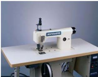
liquid and gas filters. According to Melissa Alleman, Sonobond’s vice president, a SeamMaster™ unit was recently installed at Enfilter Limited in Aberdeen, Scotland. She explains, “Enfilter is a new division of the Abenco Group and is using the Sonobond technology to bond the longitudinal seams of the liquid and gas filter cartridges it manufactures. The company
