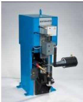
also splices tinned wires up to 35 sq. mm. using a 3500-watt power supply. It makes strong, high-quality wire connections without clipping, soldering, crimping, or dipping. The machine is perfect for producing the wire bundles found in the automotive, aircraft, computer, and consumer electronics industries. It is also used in a wide variety of other process control and industrial instrument applications.
