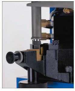
Sonobond's SpliceRite<sup>TM</sup> features specialized wire-splicing tooling to produce the lowest resistance, most reliable electrical connections possible.
