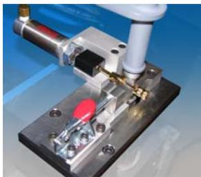
effective—soldering or mechanical methods. To accomplish this, the ultrasonic metal spot welder had to be able to hold the company's custom-designed banana plugs firmly in place so that the #10 and #12 stranded copper wires could be inserted into the back of the plug and then fused directly to the brass surface.
