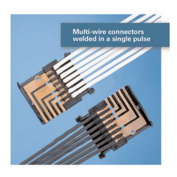
requires flat wire gang welds of 5 and 7 wires to a copper or brass terminal for a steering wheel clock spring. But the system they were using did not weld all the wires at once. They needed to repeat the process several times to achieve a finished assembly.
