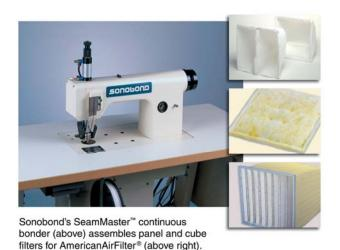
Kentucky, provides filtration products for HVAC applications, dust collection, nuclear and bio-chemical products. According to Ron Unthank, Manager, AF-Manufacturing Engineering for AmericanAirFilter, ultrasonic equipment is used to manufacture 3 of their commercial air filters.
