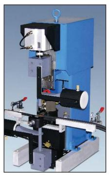
This is a dual-head SpliceRite™ system for wire splicing and metal bonding using ultrasonic waves.
