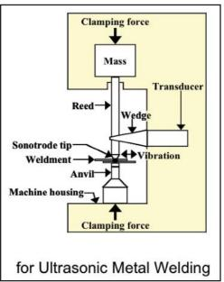
Sonobond's patented Wedge-Reed System, designed for high impedance metal welding, combines low vibratory amplitude with high vibratory force directed in a shear mode. It uses a vertical, vibrating reed, driven by a wedge-shaped coupler and transducer assembly that's perpendicular to the reed. With the line of static clamping force directly above the parts to be welded, high clamp force can be achieved without bending stress or stalling.
