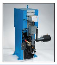
Sonobond's reliable, costeffective and environmentally friendly SpliceRite Wire Splicer welds tinned or oxidized wire bundles up to 35 square millimeters in just one pulse and without pre-cleaning.
