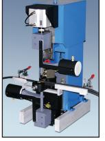
The Dual Head SpliceRite™ Wire Splicer is the first ultrasonic welder that can splice up to 100-square-millimeter wire bundles in a single pulse. It can also weld most oxidized and tinned metals.
