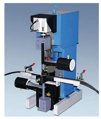
Sonobond's SpliceRite<sup>TM</sup> units provide one-pulse bare copper wire splicing of up to 100 mm<sup>2</sup> and tinned wires to 60mm<sup>2</sup>. They also feature easily changeable heat-treated, taper-lock tips capable of up to 100,000 welds and microprocessor controllers that store and recall up to 250 jobs, programming welds by height, energy or time.
