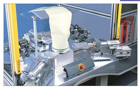
The innovative RingMasterT<sup>TM</sup> Filter Bag Machine ultrasonically attaches heavy felted filter media to rigid plastic rings, creating a dependable 360-degree bond in just two steps. The process takes less than 10 seconds and can produce up to 250 bags per hour for use in the petroleum, food, chemical and pharmaceutical and other industries.
